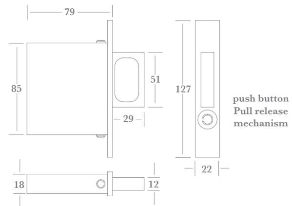
Light touch Pull retraction or automatic retraction when Pull contacts door frame.
