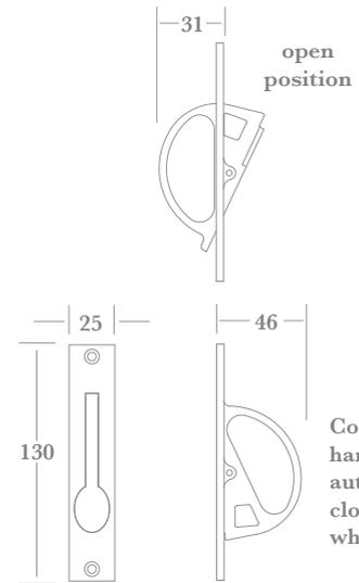
Counter-balanced handle returns automatically to closed position when released.
