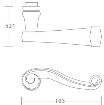
\* total projection: add 7mm for rosette, 6mm for backplate with flush collar & 10mm for plate with raised collar.
