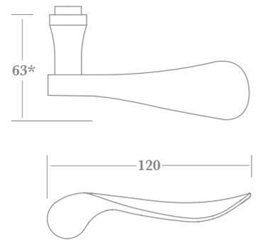
\* total projection: add 7mm for rosette, 6mm for backplate with flush collar & 10mm for plate with raised collar.
