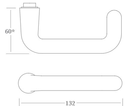
\* total projection: add 7mm for rosette, 6mm for backplate with flush collar & 10mm for plate with raised collar.
