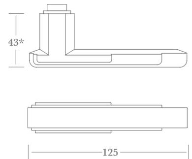
\* total projection: add 7mm for rosette & 6mm for backplate. Lever design is suitable for use with backplates fitted with either type G flush collar or type J raised collar (other raised collar designs are not recommended).
