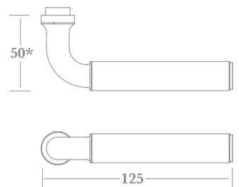
\* total projection: add 7mm for rosette, 6mm for backplate with flush collar & 10mm for plate with raised collar.
