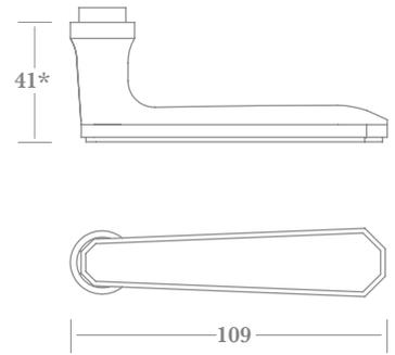
\* total projection: add 7mm for rosette, 6mm for backplate with flush collar & 10mm for plate with raised collar.
