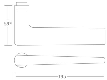
\* total projection: add 7mm for rosette, 6mm for backplate with flush collar & 10mm for plate with raised collar.
