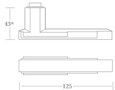
\* total projection: add 7mm for rosette & 6mm for backplate. Lever design is suitable for use with backplates fitted with either type G flush collar or type J raised collar (other raised collar designs are not recommended).
